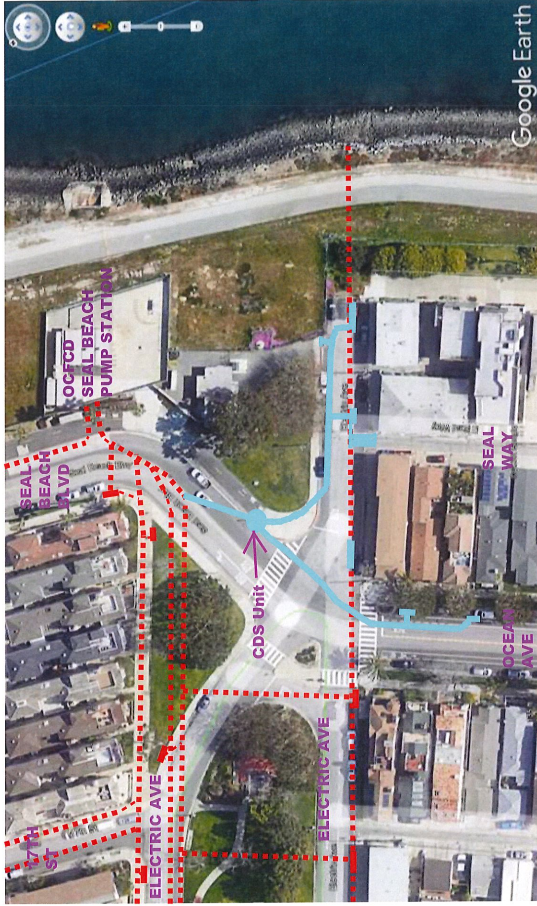
Figure 2 – Proposed Storm Drain Facility
